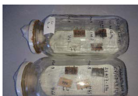
Figure 1: Screening test samples after 6 weeks decay by Coriolus Versicolor
