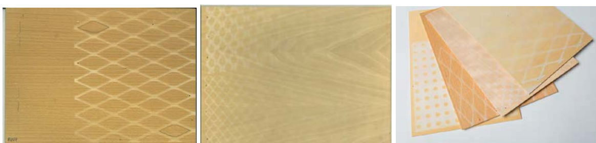
Figure 1: Samples of UV-modification on poplar and beach wood by using different mesh masks and samples with the special transition pattern thanks to inclination of the mask.
