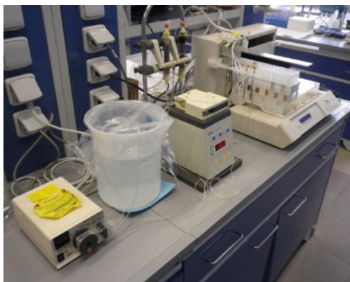
Complete column-leaching set-up in operation;
