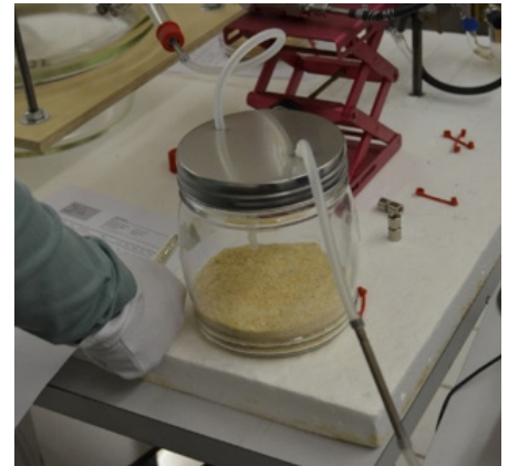
Glass container with wood dust and the sampling tubes. In the back is the clean air supply tube and in the front is the tenax tube attached to container. The other end of tenax tube is attached to a pump.
