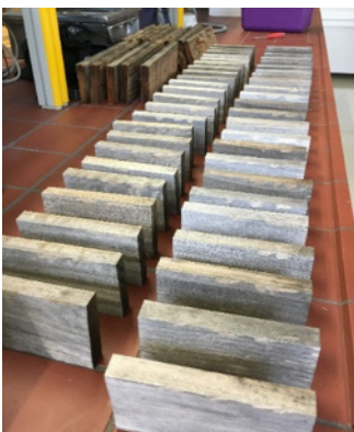
Carolina and Eucalyptus globulus samples on the first day the samples were set up on the rooftop of the university building for the weathering experiment;
