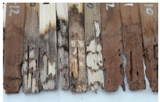
Samples after 3 months of termite exposure
