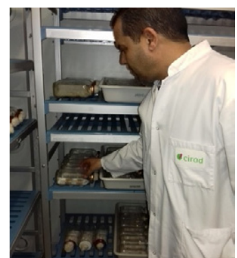
Preparation of fungal resistance screening tests. Photo credit - Kévin Candelier
