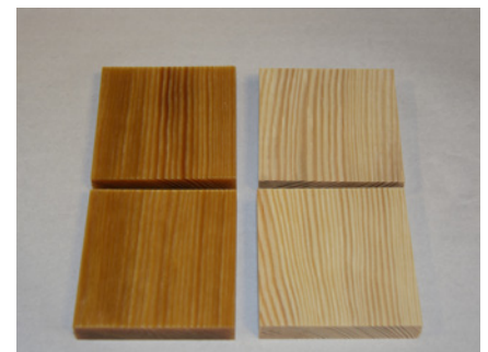
Wood samples treated with chemically modified lampante oil (left) and untreated wood samples (right).
