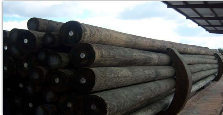
Wooden posts (pine) treated with creosote
