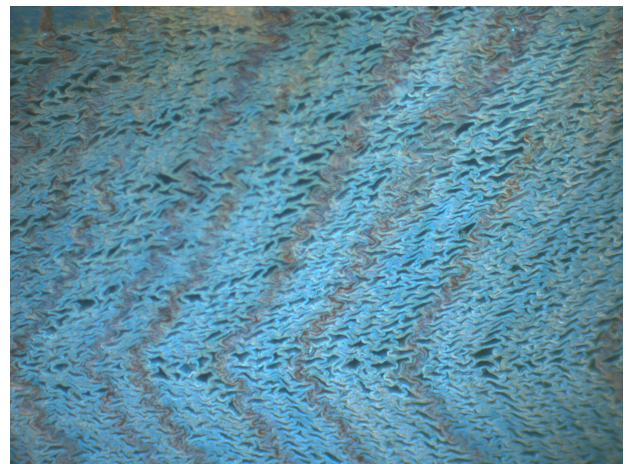
Figure 1: Cross section of hybrid poplar densified with THM treatment at 160°C under a saturated steam environment.
