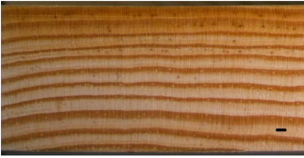
Figure 2: Cross section of surface densified pine wood.
