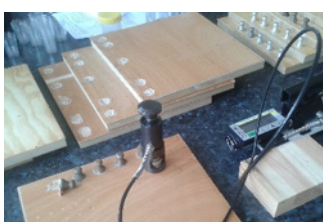
DeFelsko PosiTest Pull-off Adhesion Tester for determining of the adherence of lacquer coatings
