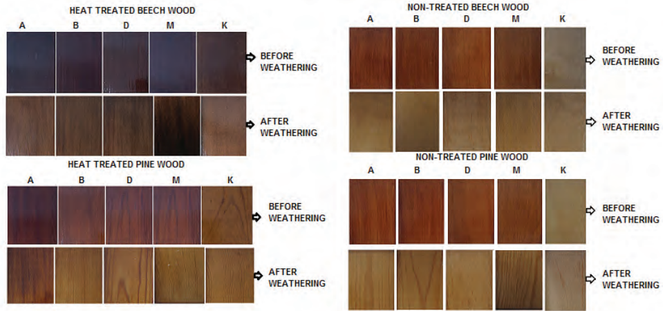
Figure 1: Macroscopic evolution of waterborne acrylic coating systems applied to beech and pine wood before and after artificial weathering test (A: black pine; B: calabrian pine; D: alder; M: oak; K: control).
