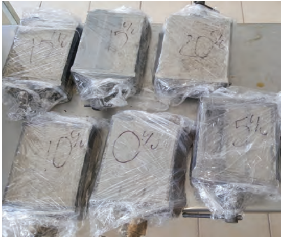
Figure 1: The samples of wood sawdust and alkali activated slag bio-composite
