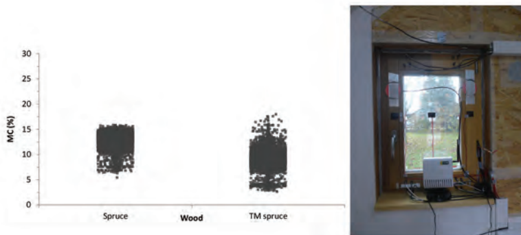
Figure 2: Moisture content distribution in the window (right) made of non-modified spruce and thermally modified wood in Ljubljana. On every location, 12.000 measurements were performed in the period between October 2013 and October 2018.
